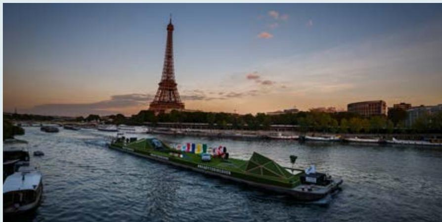
"We filled the 11m wide barge with 1,800 tons of earth, to get the correct trim for the design specification. The production weighed about 200 tons, including 60 tons of water for the pool, and was by no means equally distributed. Keeping the balance across both the longitude and transverse was absolutely critical," Star Events' Project Manager, Gavin Scott, says.
